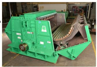
Hydraulic doors make accessing critical wear parts easy.
